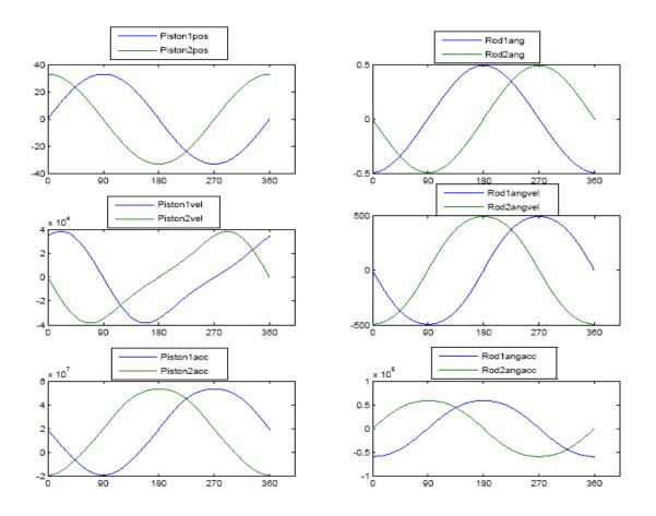
In the above plots, the horizontal axis is the crank angle, in degrees. The vertical axis in the top plots are position form midstroke in mm on the right and radians on the left. The middle plots are mm/sec and radians/sec. The lower plots are mm/sec/sec and radians/sec/sec.
