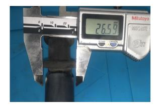
The seal needs to be aprox 24~25mm wide but rely in test fitting not measurements
